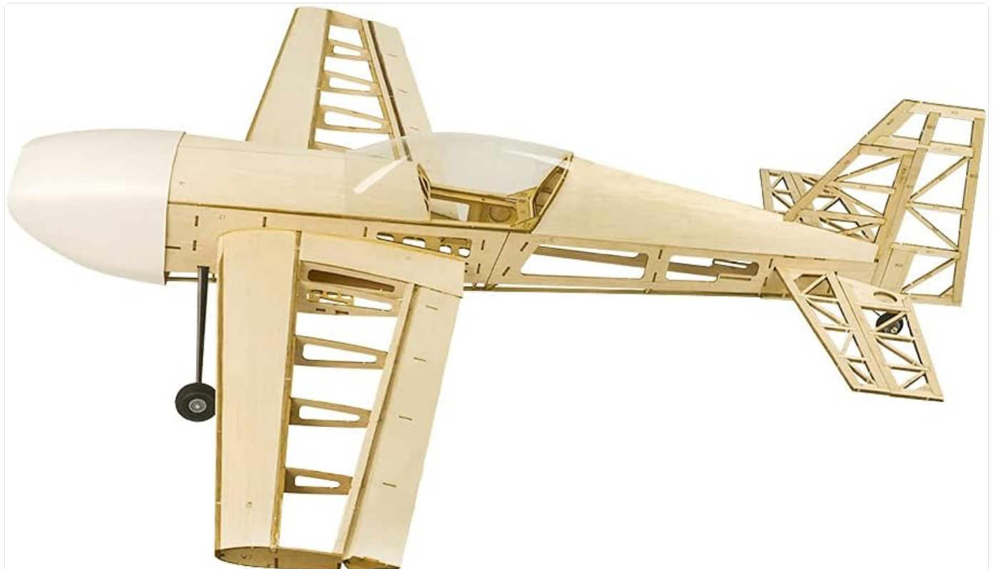
Image 4.2: Side view of the assembled EXTRA330 RC airplane, showcasing the complete airframe structure before covering.
