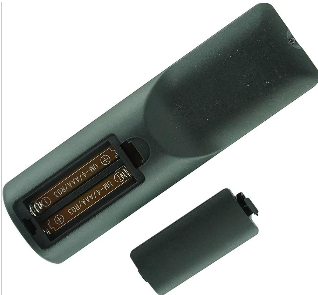
Image: Back of the remote control with the battery cover removed, illustrating the correct orientation for AAA battery insertion. Note the positive and negative terminals.
