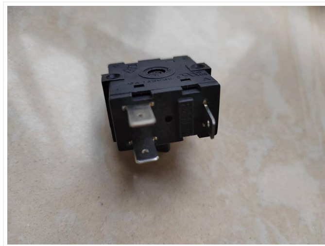
Figure 3.3: Angled view of the rotary switch, providing a clearer perspective of its compact design and terminal layout.
