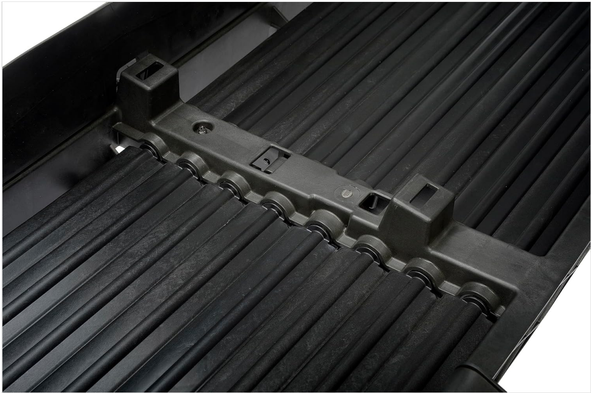
Figure 5: Detailed view of the shutter slats and their pivot points, which control airflow.
