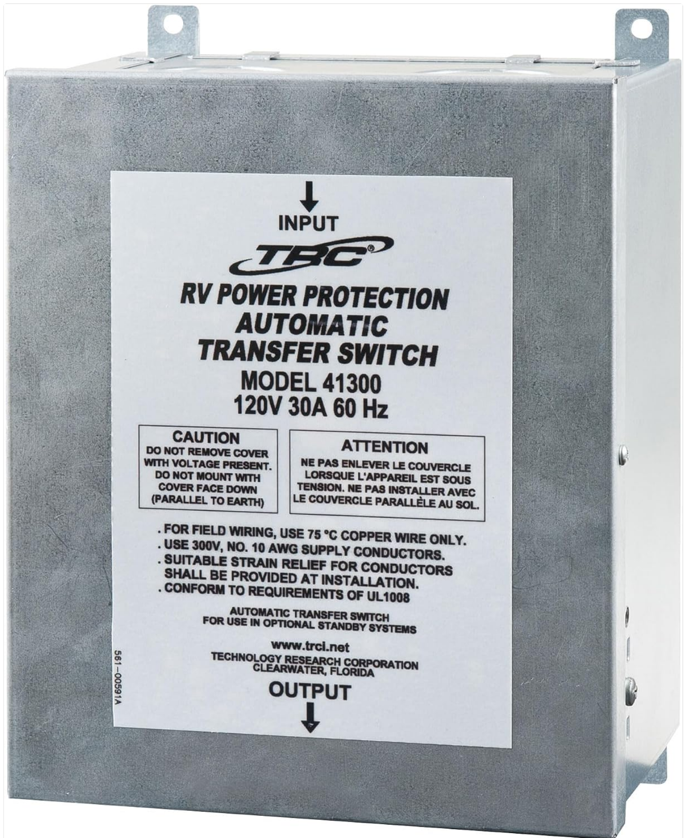
Image of the Southwire 41300 Hardwire Automatic Transfer Switch. The front label indicates it is an RV Power Protection Automatic Transfer Switch, Model 41300, 120V 30A 60 Hz. It also displays caution notes regarding voltage presence, mounting orientation, and wiring requirements, including the use of 75°C copper wire and 10 AWG supply conductors.
