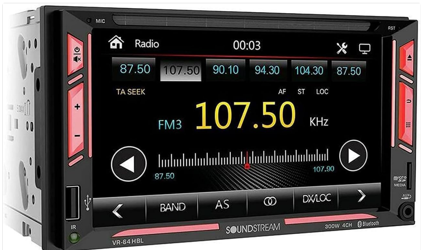
Figure 4: The radio interface of the VR-64HBL, showing the current FM frequency (107.50 MHz), station presets, and controls for tuning and band selection.
