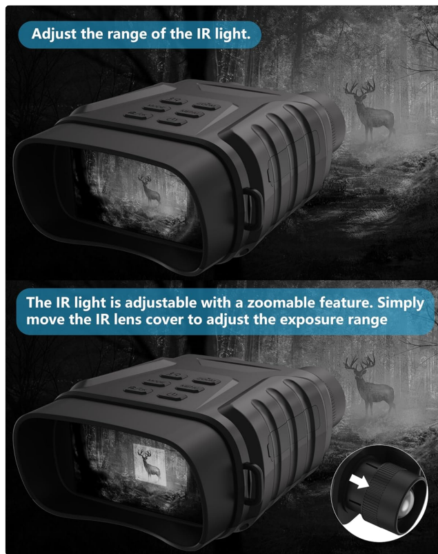
Figure 5: Adjusting the IR light range by moving the IR lens cover allows for precise exposure and enhanced clarity of distant objects in darkness.
