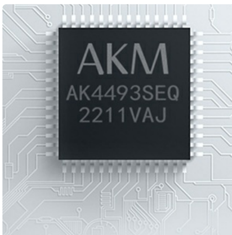
Image: Close-up of the AK4493S DAC chip, central to the E30II Lite's audio processing.
