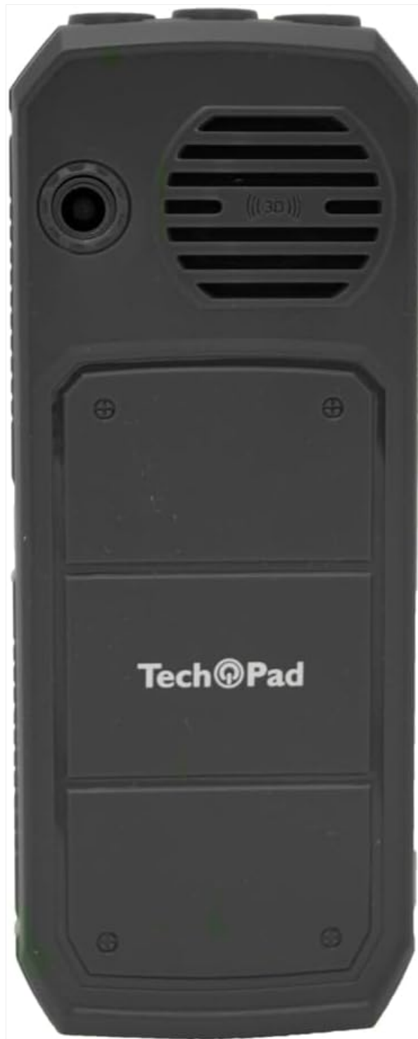
Image 2: Rear view of the TECH PAD P62 Feature Phone, showing the speaker grille, headphone jack, and the textured back cover with the "Tech Pad" logo. This area typically houses the battery and SIM/memory card slots.
