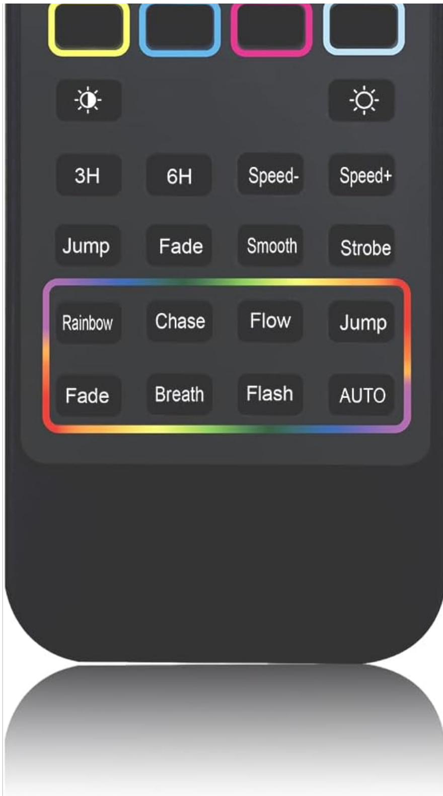
Image 1: Front view of the NOVOSTELLA RF Remote Control, displaying its various buttons for power, color selection, timing, speed adjustment, and dynamic lighting effects.
