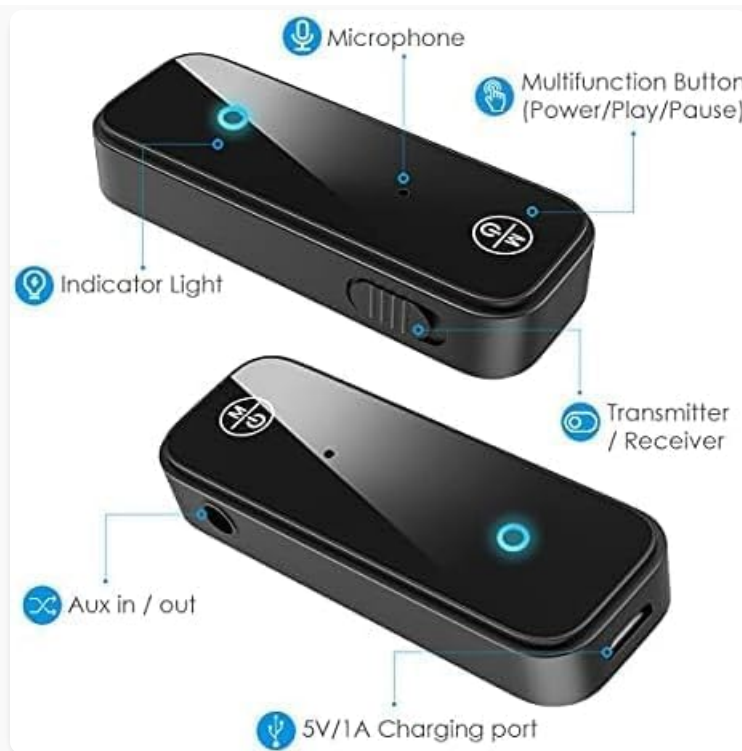
Figure 3: Labeled diagram of the Ankilo Bluetooth adapter. Key components include the Microphone, Multifunction Button (Power/Play/Pause), Indicator Light, Transmitter/Receiver (TX/RX) switch, Aux in/out port, and 5V/1A Charging port.
