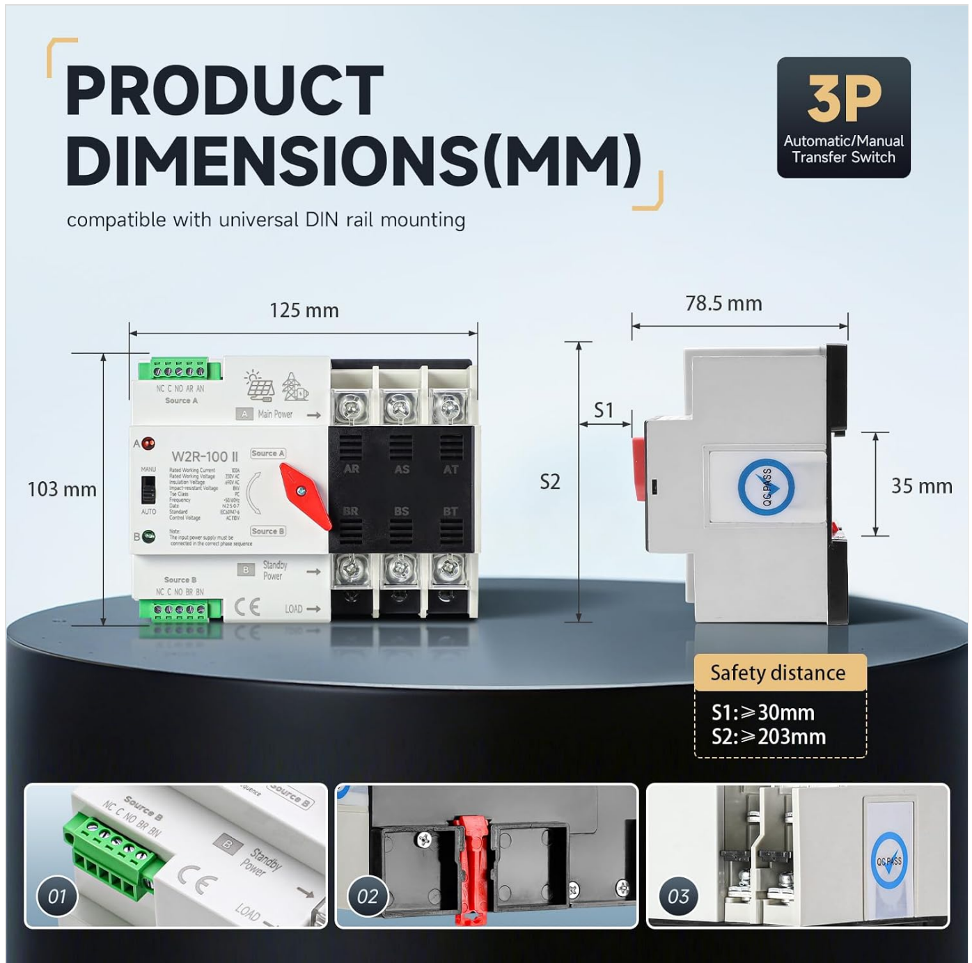
Figure 6: Product Dimensions (in mm)
