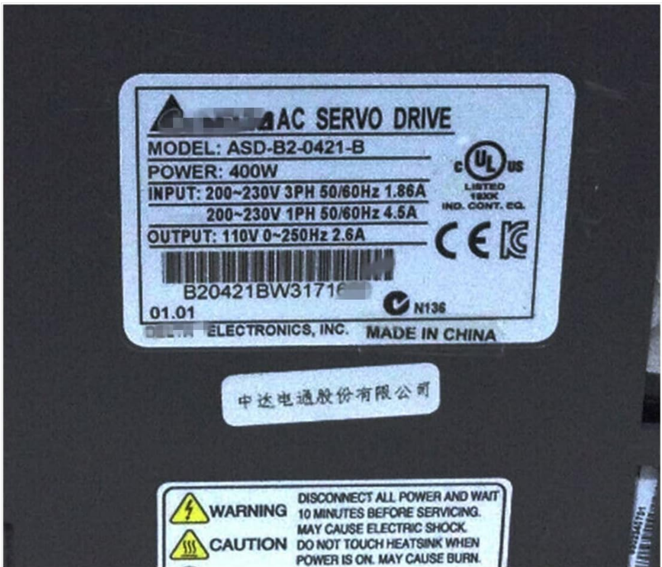
Figure 2.1: Product label with electrical specifications and safety warnings. Note the warnings regarding disconnecting power before servicing and avoiding contact with the heatsink.
