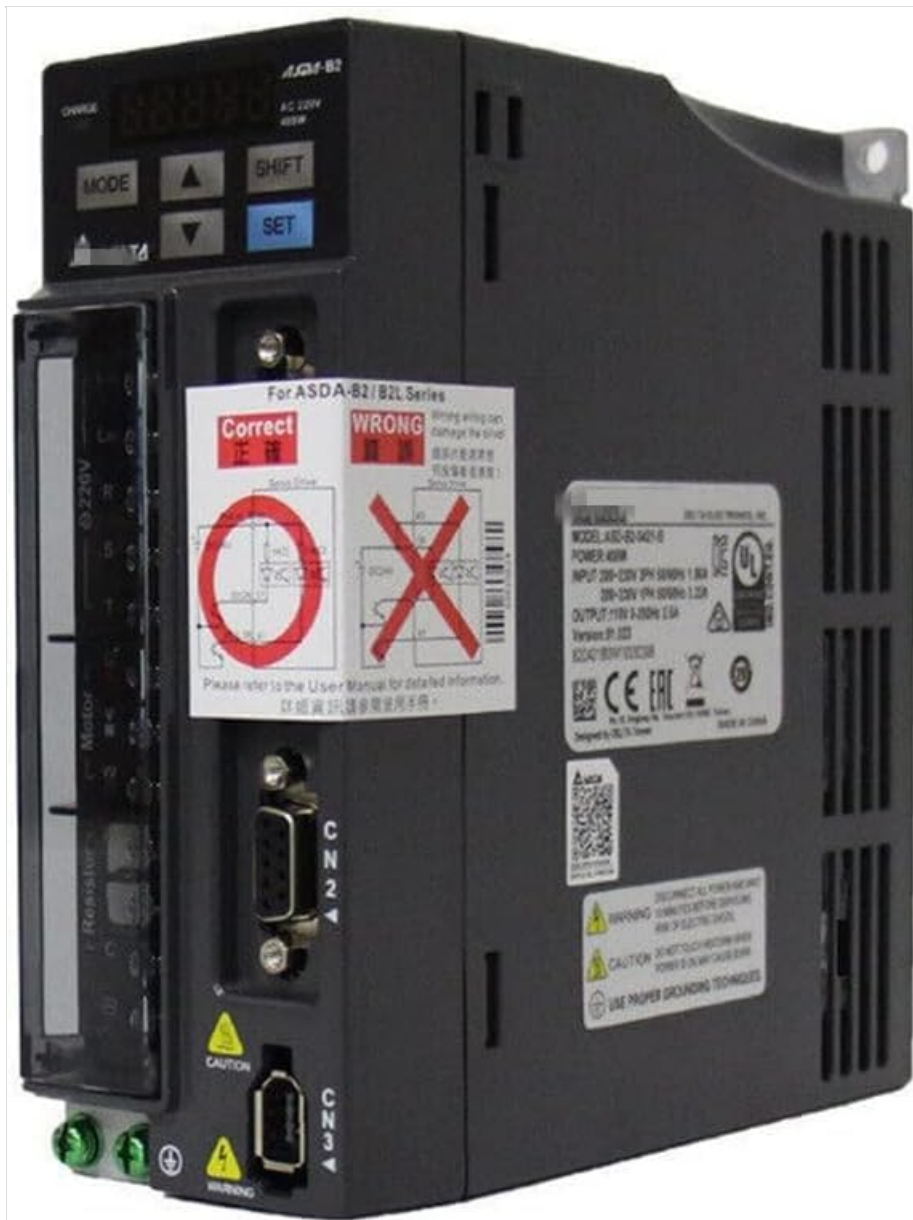
Figure 5.1: Servo drive with visible connection ports and a wiring diagram. Pay close attention to the "Correct" and "Wrong" wiring examples provided on
