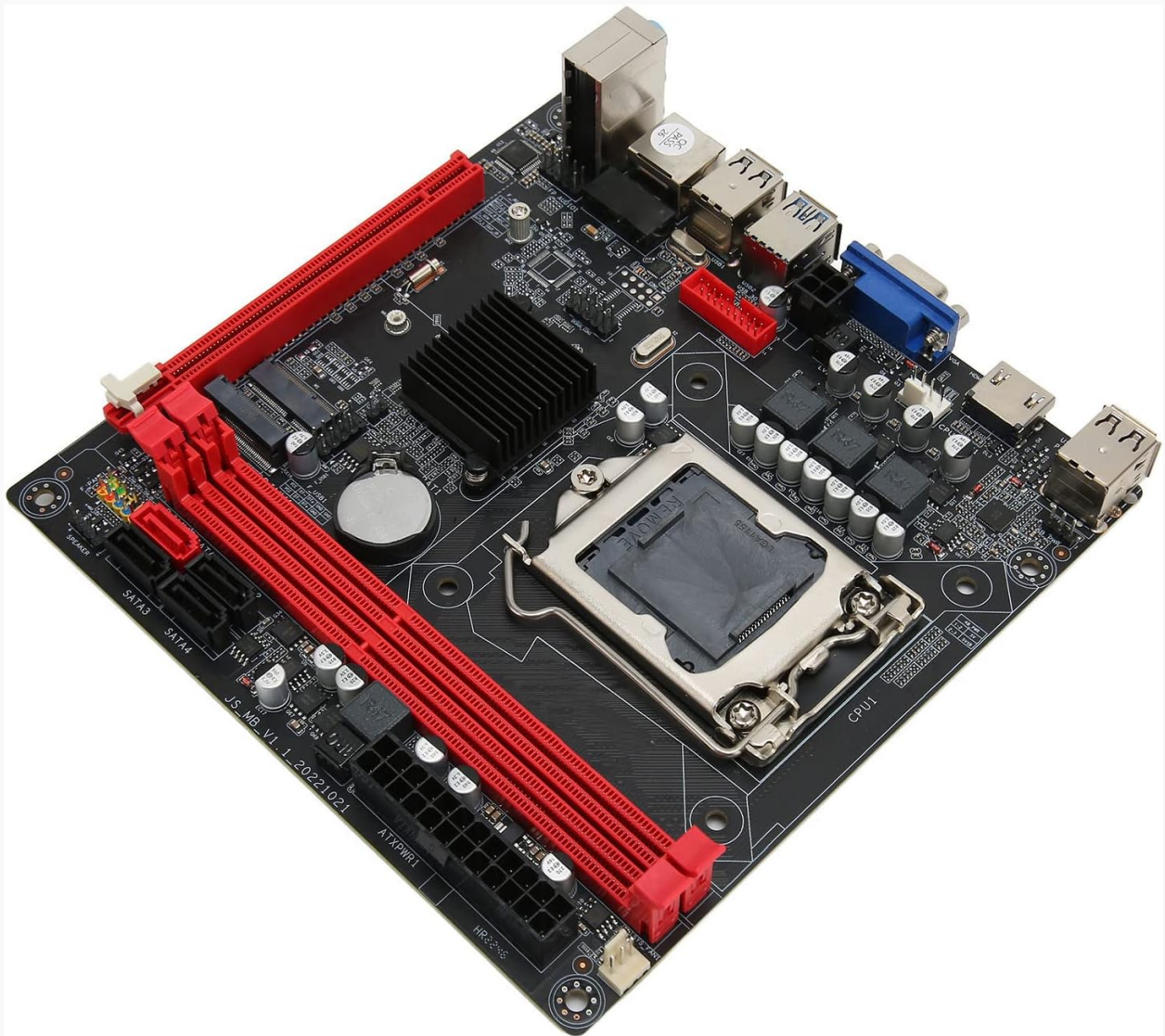
Figure 1: Top-down view of the Cuifati ATX B75A Motherboard, showcasing the CPU socket, DDR3 memory slots, PCIe slot, and various ports.
