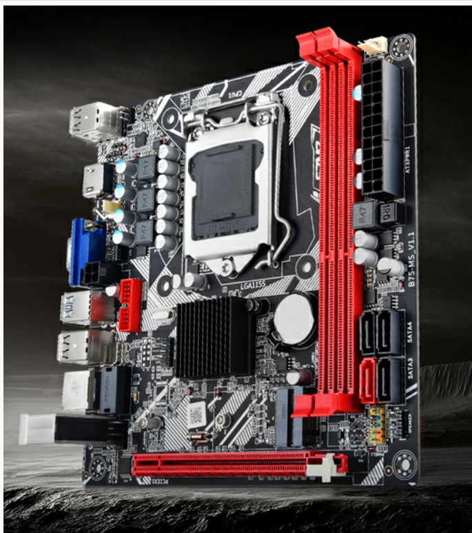
Figure 1: Top-down view of the Cuifati ATX B75A Motherboard, showcasing the CPU socket, DDR3 memory slots, PCIe slot, and various ports.
