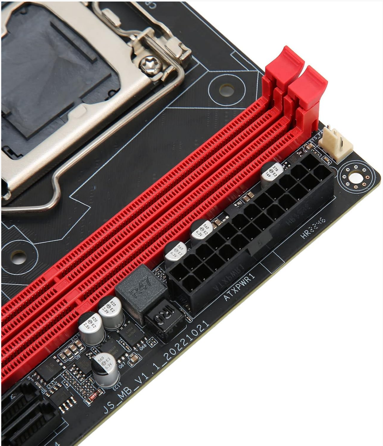
Figure 6: Close-up view of the DDR3 memory slots and the 24-pin ATX power connector, essential for RAM and main power connections.
