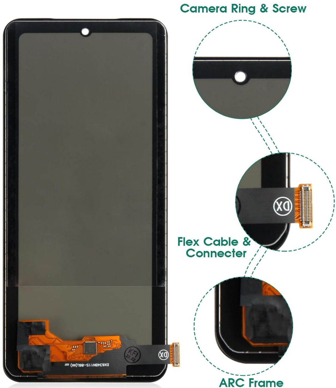
Image 2: Close-up view of the flex cable and connector, highlighting critical connection points for installation.
