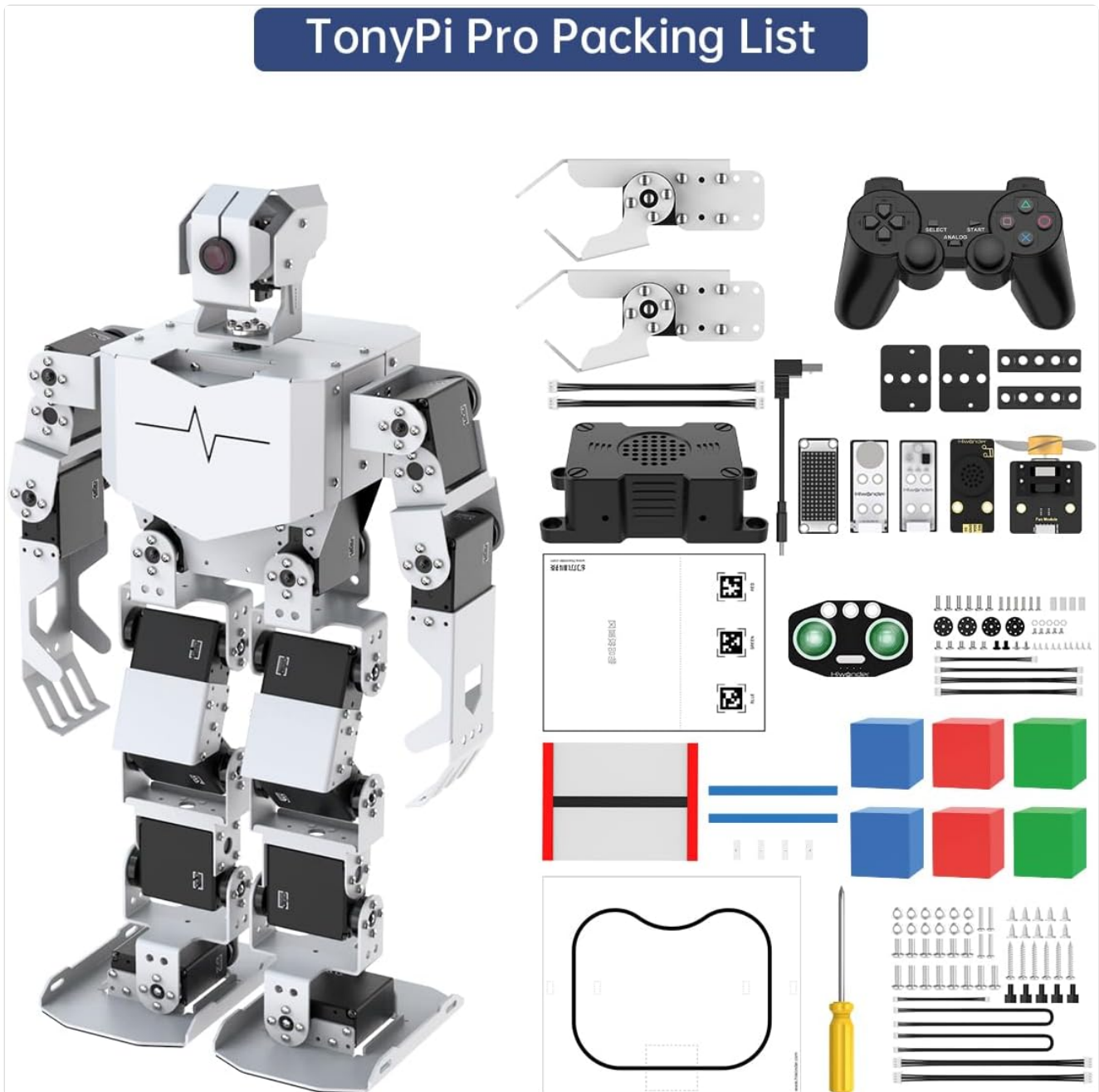
Figure 3: Visual representation of the TonyPi Pro Kit contents, including robot parts, controller, and accessories.
