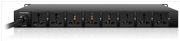
Figure 5.2: Rear view of the Sound Town STPS-1028, illustrating the 8 sequenced universal outlets and the main AC input.
