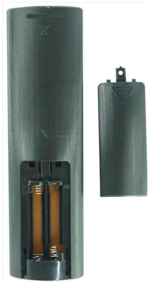
Figure 2.1: Back of the remote control with the battery cover removed, illustrating the correct orientation for AAA battery insertion.
