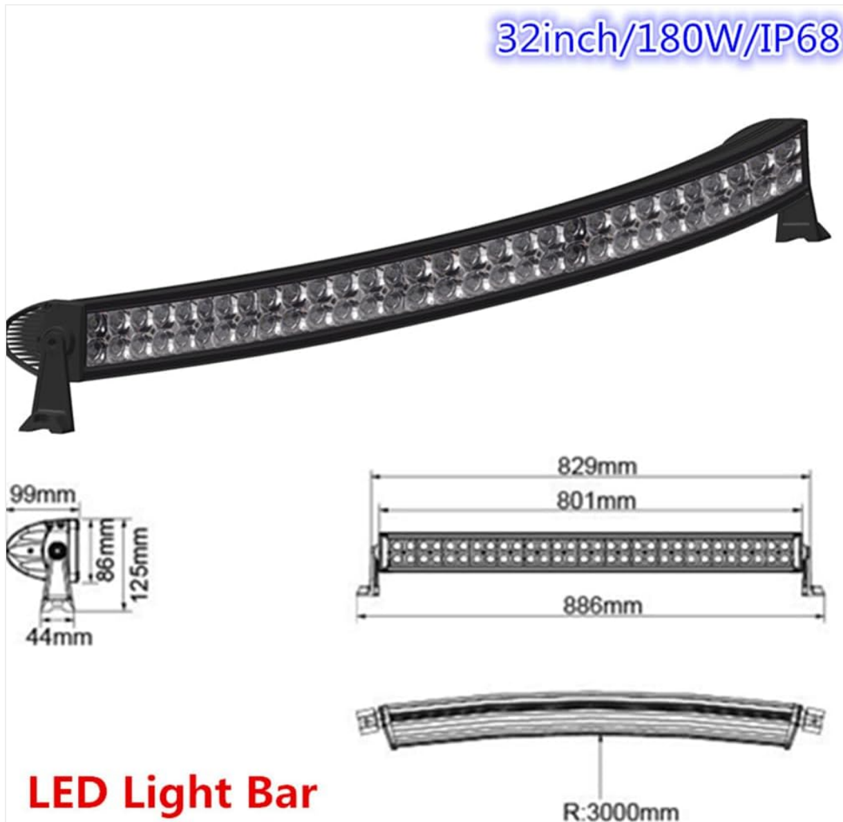
Figure 2: Dimensional drawing of the LED Light Bar, showing key measurements.
