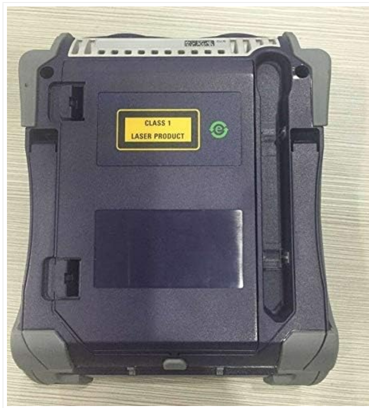
Figure 2.1: Rear view of the Smart OTDR, highlighting the Class 1 Laser Product warning label.
