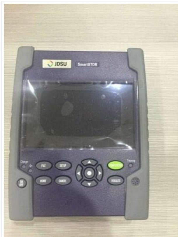
Figure 1.1: Front view of the JDSU VIAVI Smart OTDR, showing the display and control buttons.
