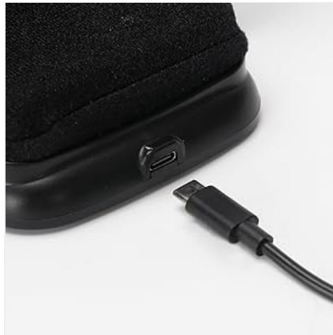
Image: The Type-C USB charging port located on the device.
