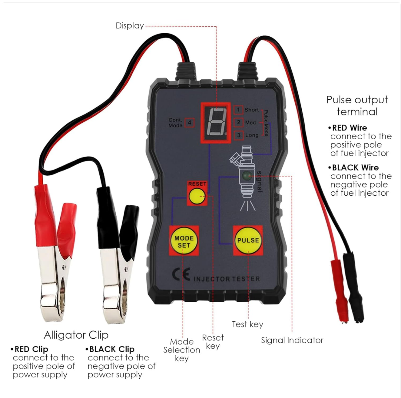
Figure 3.2: Labeled diagram of the injector tester's components.
