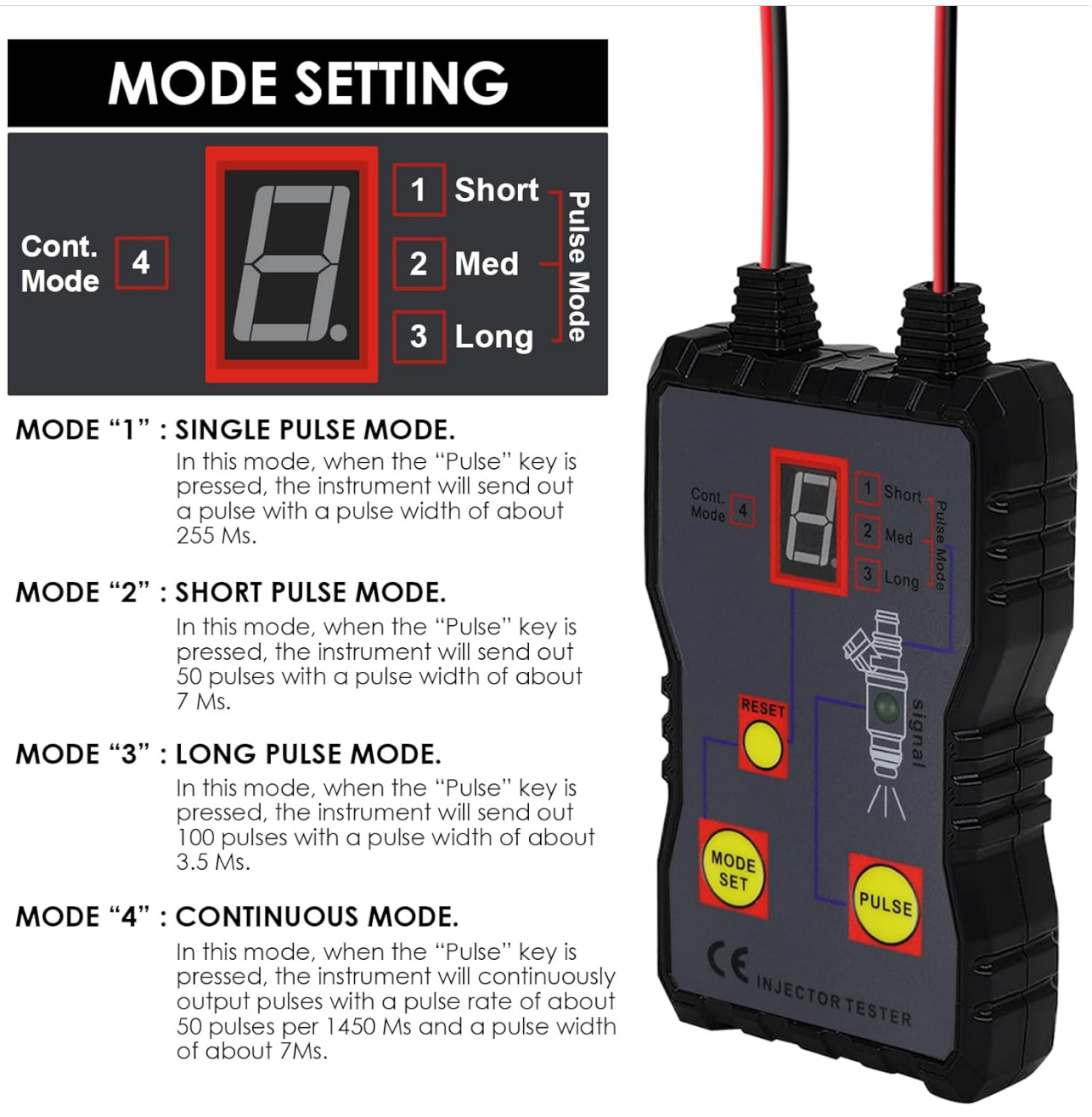
Figure 5.1: Detailed explanation of the four pulse modes.
