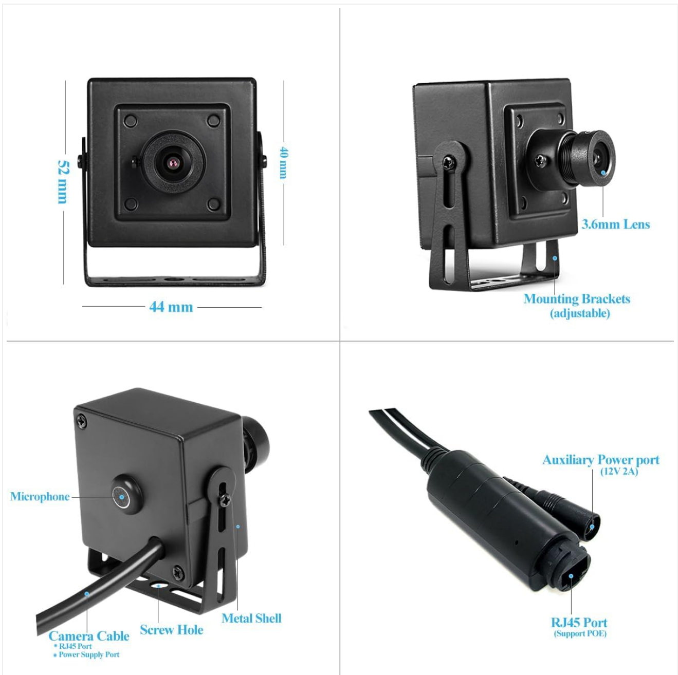
Image 3.1: This image illustrates the camera's dimensions (52mm height, 44mm width, 40mm depth) and highlights key components such as the 3.6mm lens, microphone, mounting brackets, RJ45 port (for POE), and auxiliary 12V 2A power supply port.
