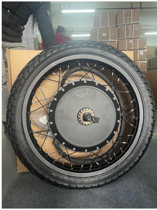
Image 3.1: QS 273 8000W Motorwheel with Terrain Tire. This image shows the complete motorwheel assembly, including the hub motor, spokes, rim, and a knobby terrain tire.
