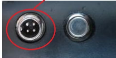
Figure 3.2: Compatibility check for the charger. This diagram illustrates the difference between a compatible 3-prong female connector and an incompatible 4-prong female connector, emphasizing the importance of verifying your device's port type.
