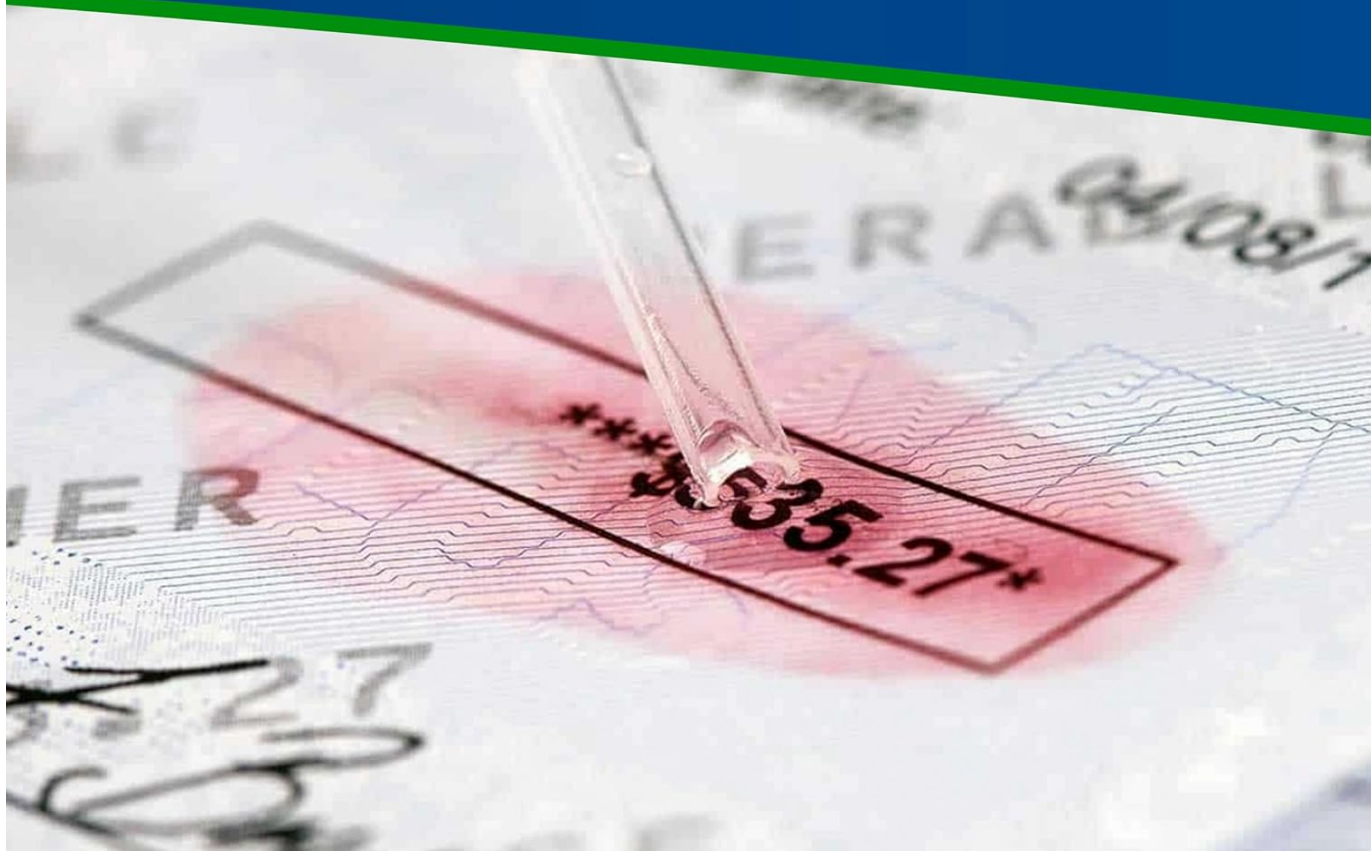
Figure 5: A close-up view illustrating the TROY MICR Toner Secure's anti-tamper feature, where a bright red stain permeates the document upon attempted chemical alteration, indicating fraud.
