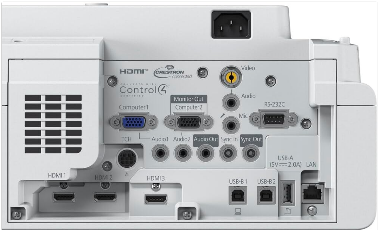
Figure 4.3: Rear panel connections of the BrightLink 760Wi.
