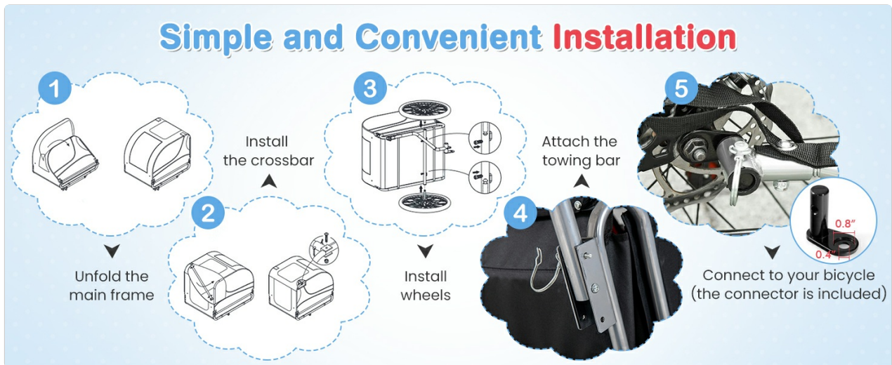
Image 2.1: Step-by-step diagram illustrating the assembly process of the pet bike trailer.
