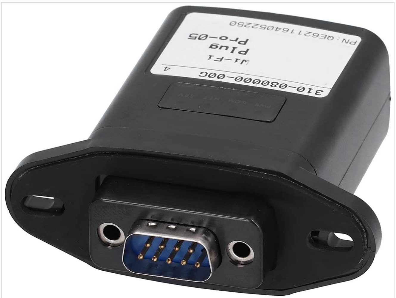
Image 3.2: The RS232 communication port on the Wi-Fi module where the connecting cable is inserted.
