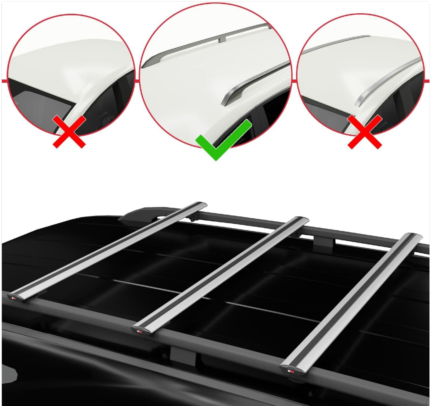
Image: Visual guide illustrating the correct type of roof rail for compatibility (roof rails with a gap).
