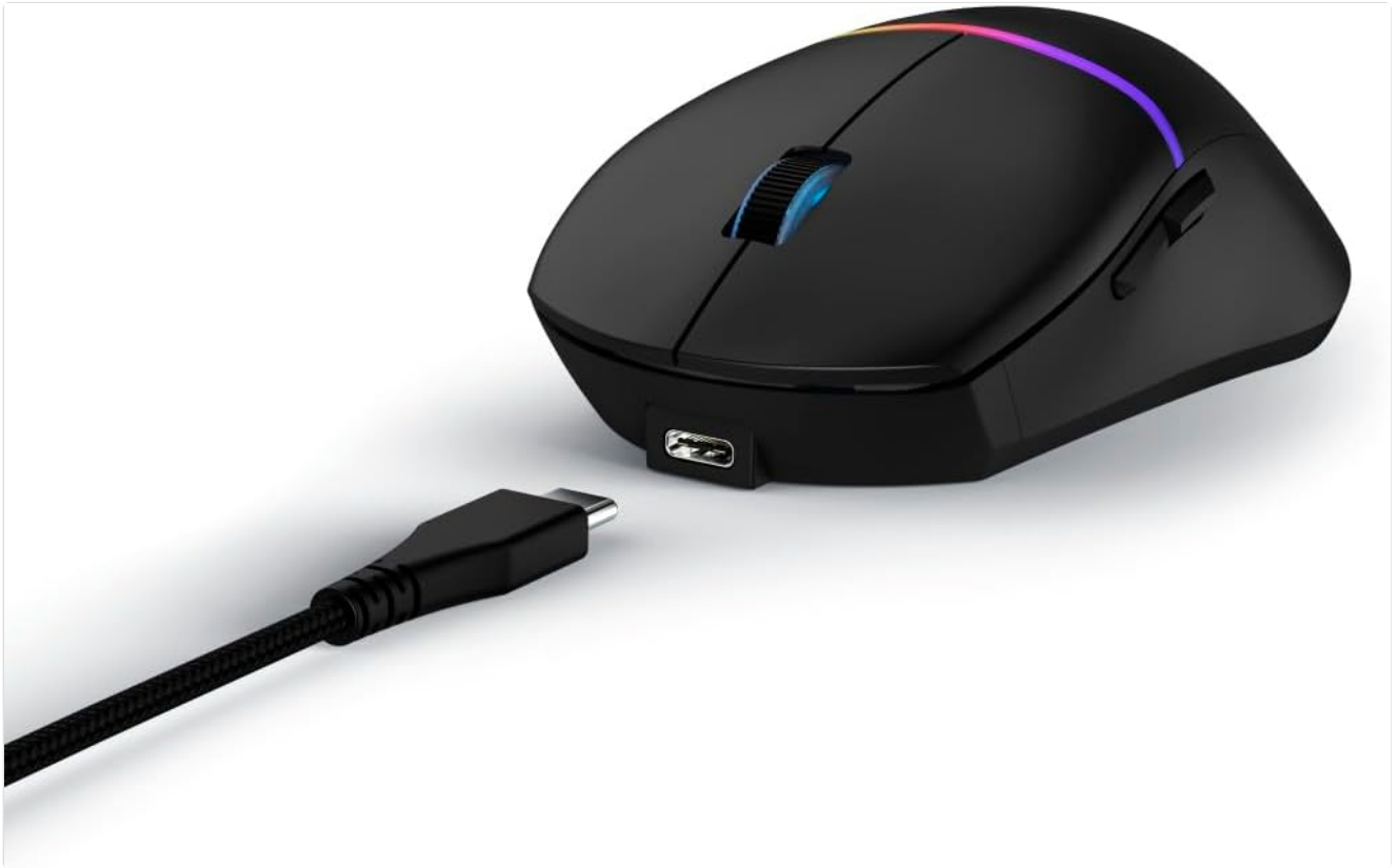
Image: The uRage Reaper 330 gaming mouse with its detachable USB-C cable, illustrating the connection point.
