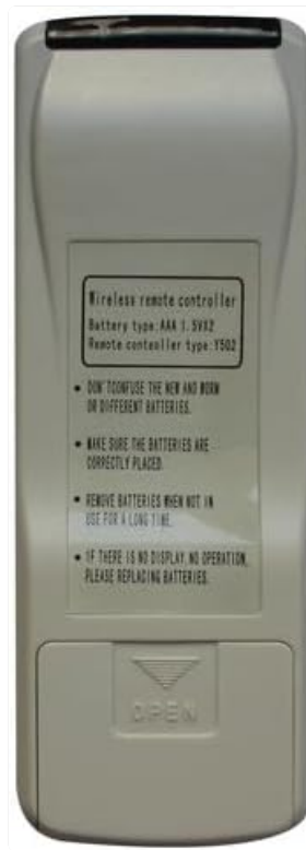
Image 2.1: Back of the remote control with the battery compartment. The compartment cover is located at the bottom, designed to slide open for battery insertion.
