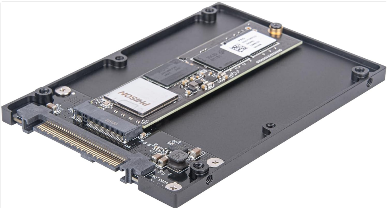
Image: An M.2 NVMe SSD correctly installed and secured within the MUA01 adapter, ready for enclosure assembly.
