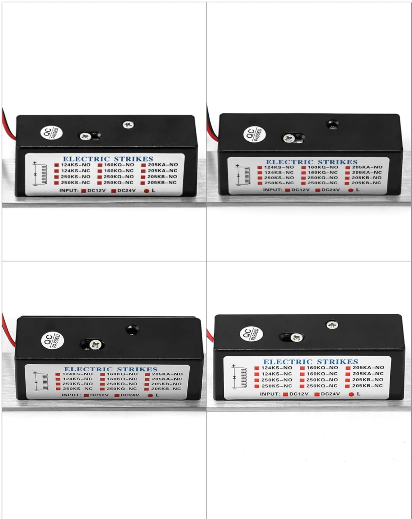
Image 6.1: Rear view of the electric strike, highlighting the screw for switching between Fail-Safe (NC) and Fail-Secure (NO) modes, along with voltage selection.
