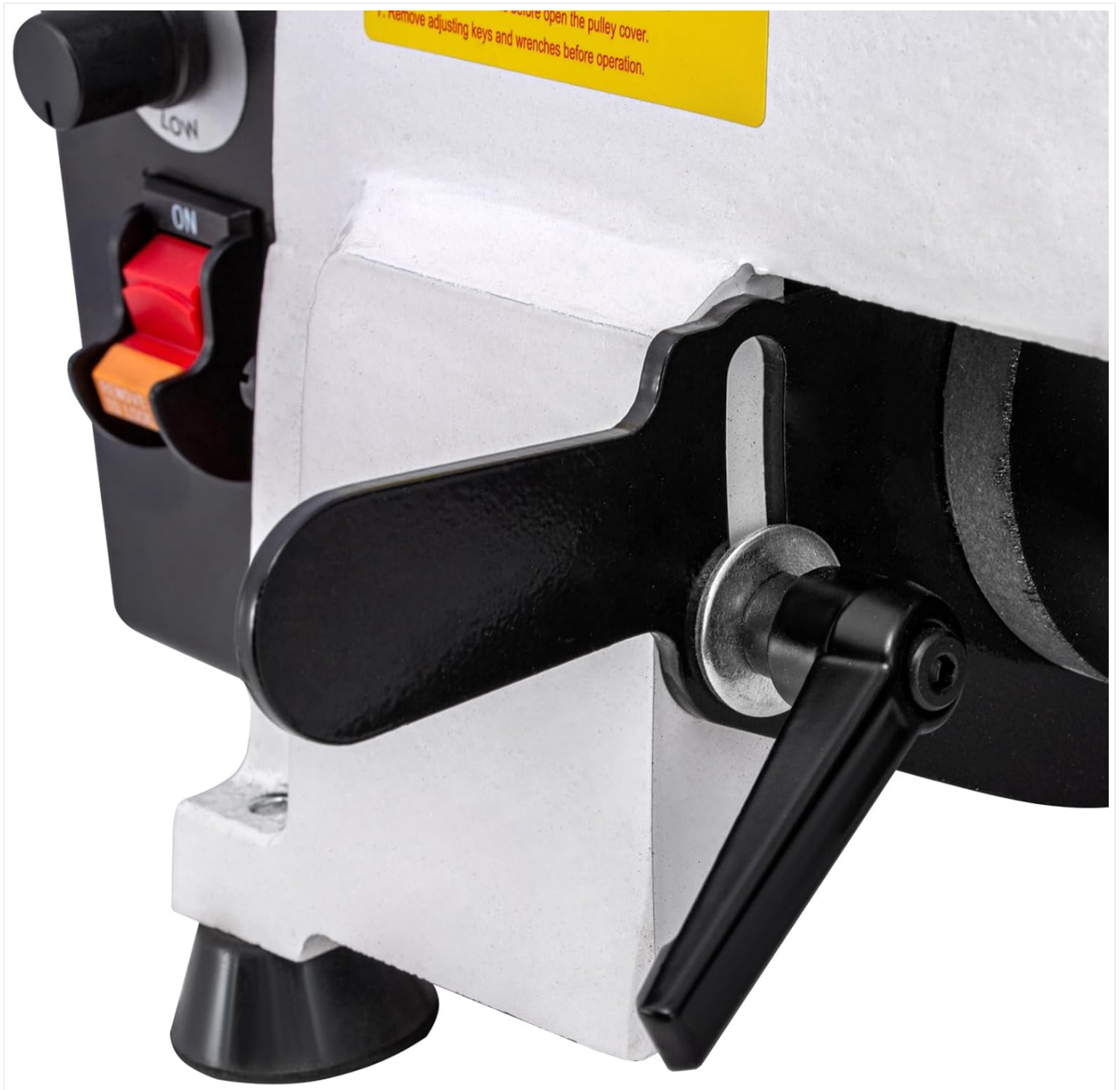
Figure 3.1: Detail of the tool rest locking mechanism, showing how to secure it to the lathe bed.
