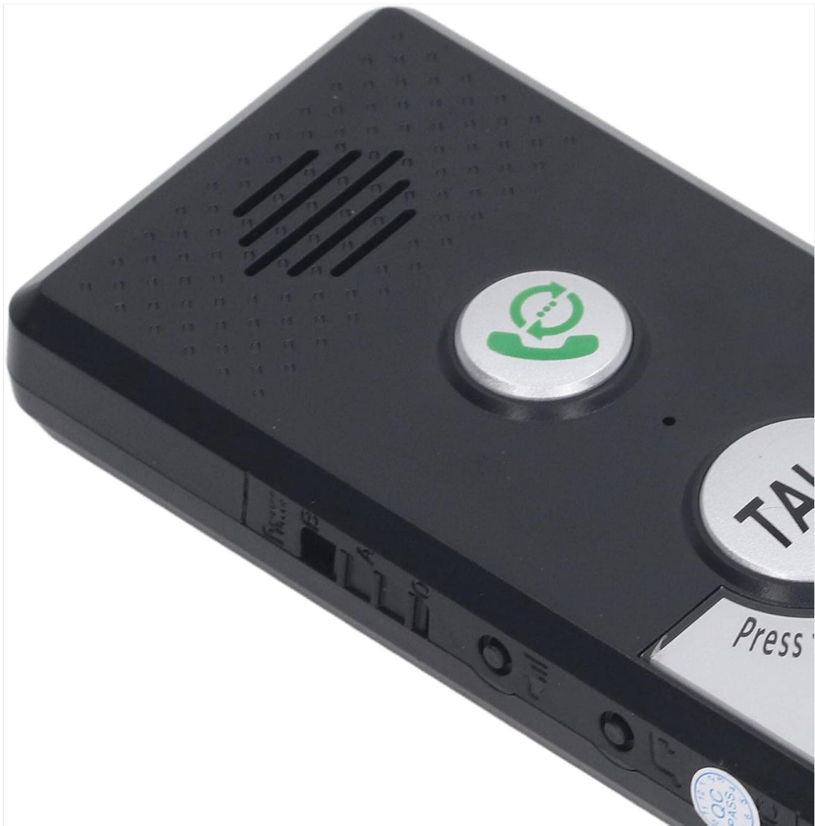
Image: A close-up of the Naroote H8 intercom unit, showing the speaker grille and the green call button, which can be used for initiating calls or as a doorbell function.
