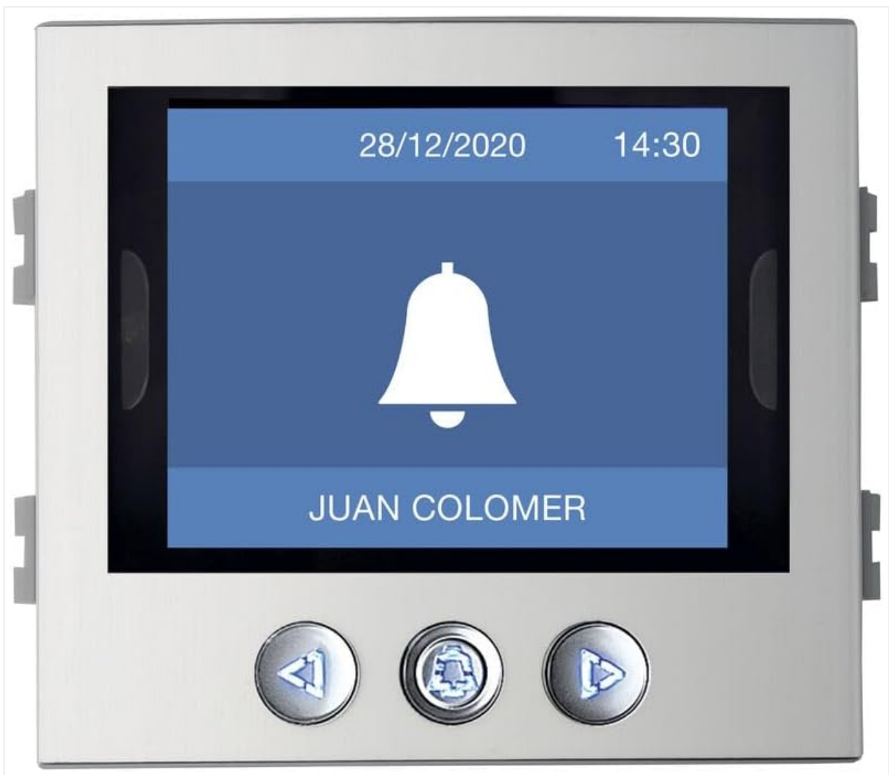
Figure 2.1: Front view of the FERMAX DUOX Plus Skyline Display 7470. The screen displays a notification with a bell icon and a name, while three circular buttons are located below for user interaction.
