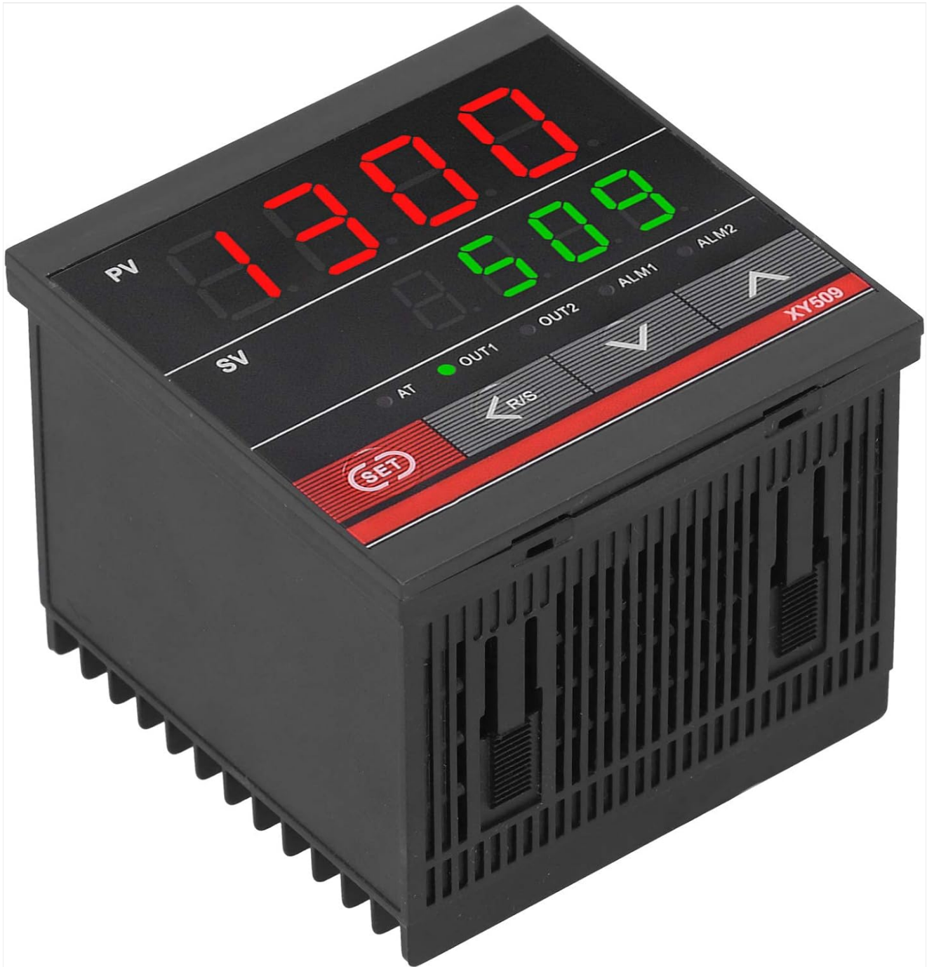
Figure 1: Front View of XY509 Controller. This image shows the front panel of the Dilwe XY509 PID Temperature Controller, featuring the red PV (Process Value) display, green SV (Set Value) display, and control buttons including SET, R/S, and arrow keys for navigation and adjustment. Indicator lights for AT (Auto-Tune), OUT1, OUT2, ALM1, and ALM2 are also visible.
