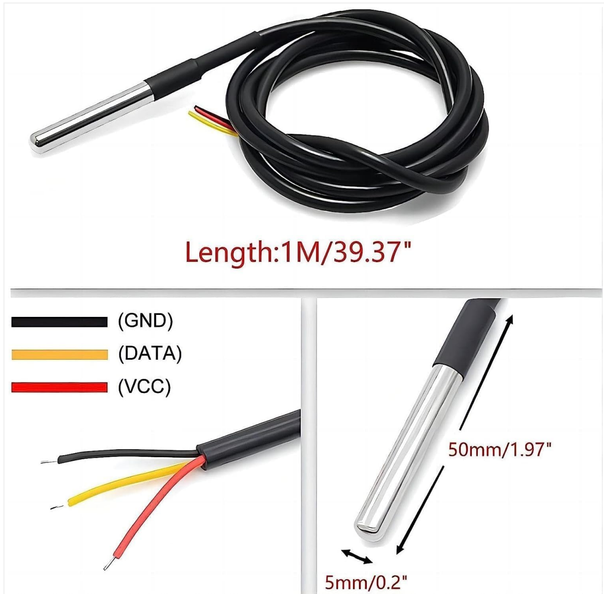
Image 3: This image displays the wiring diagram for the DS18B20 sensor, indicating Red (VCC), Yellow (Data), and Black (GND) connections. It also shows the physical dimensions of the probe.
