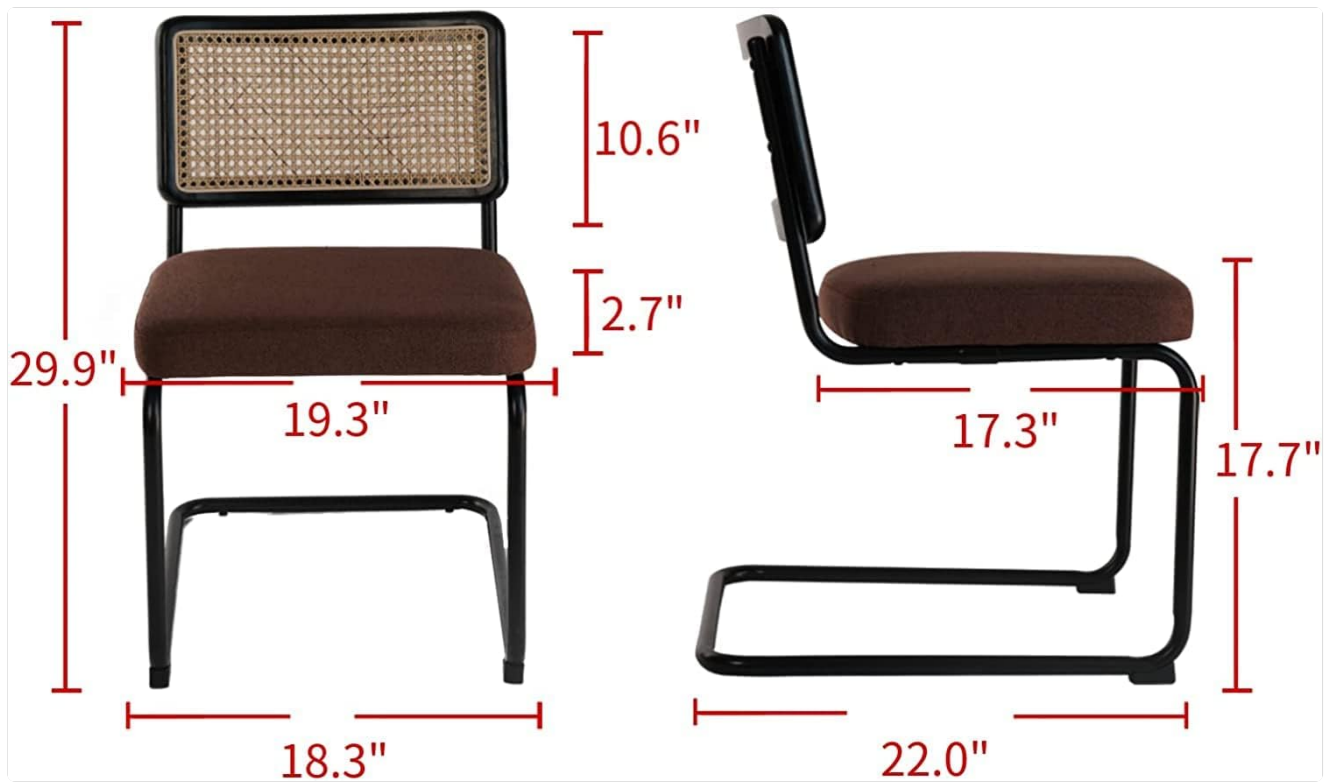
Image: Dimensional diagram of the chair, useful for understanding component placement during assembly.
