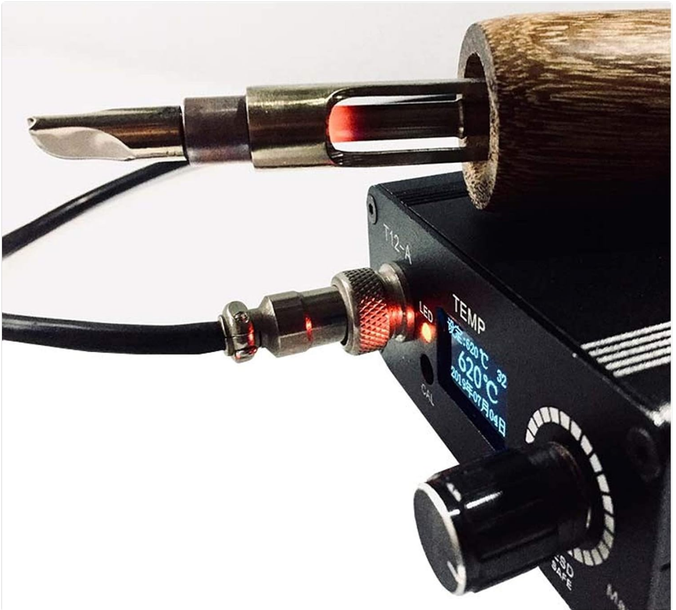
Image: Close-up of the hand-held tool with a hot head attached, connected to the control unit. The display shows the current temperature.
