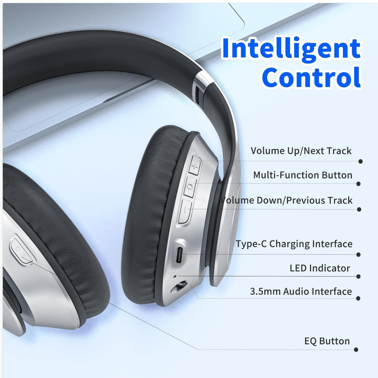
Image: Detailed view of the Uliptz WH203A headphone controls, including volume buttons, multi-function button, charging port, LED indicator, 3.5mm audio jack, and EQ button.
