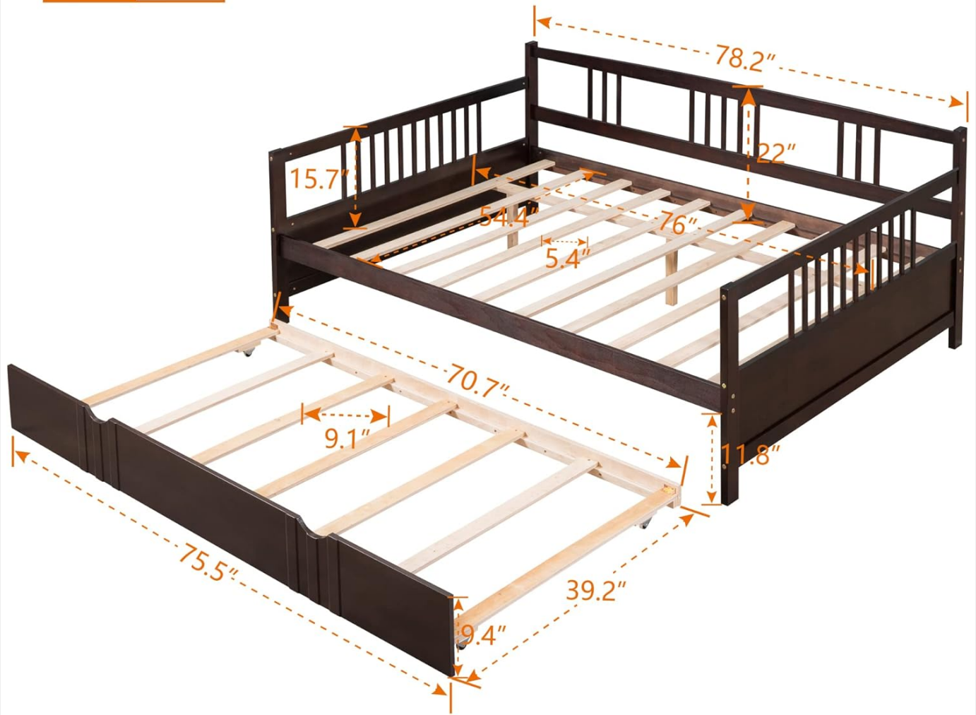
Figure 3.1: Dimensional diagram of the Polibi Full Size Daybed and Twin Trundle.
