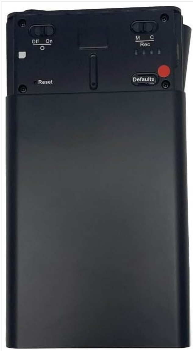
This image displays the back panel of the Lawmate PV-PB30W, revealing the hidden controls including the power switch, reset button, and recording mode selectors. The SD card slot is typically located near these controls.
