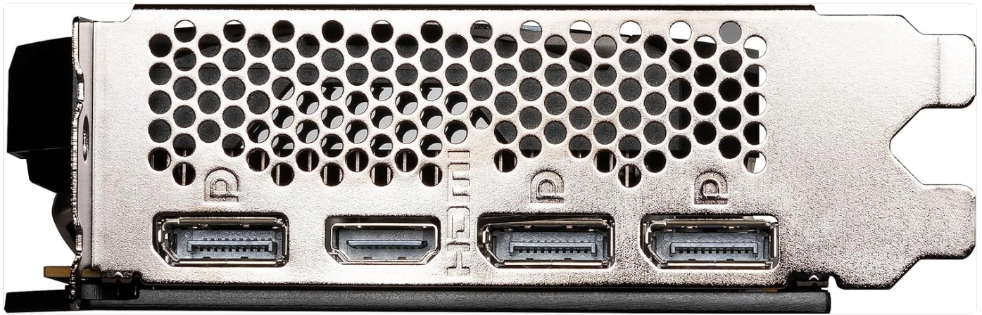
Image: Close-up of the display output ports on the MSI GeForce RTX 4060, including DisplayPort and HDMI connections.
