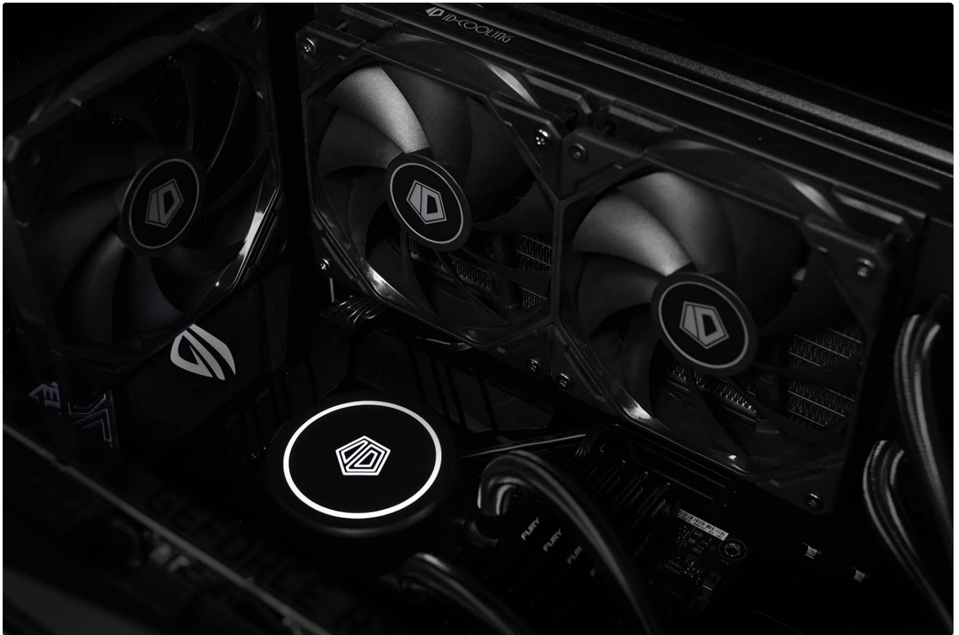
Figure 6: The 240mm radiator with its two 120mm PWM fans installed.
