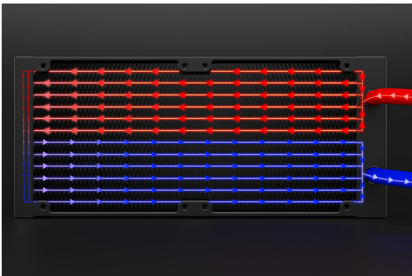
Figure 3: Diagram illustrating the efficient heat dissipation process within the 240mm radiator.
