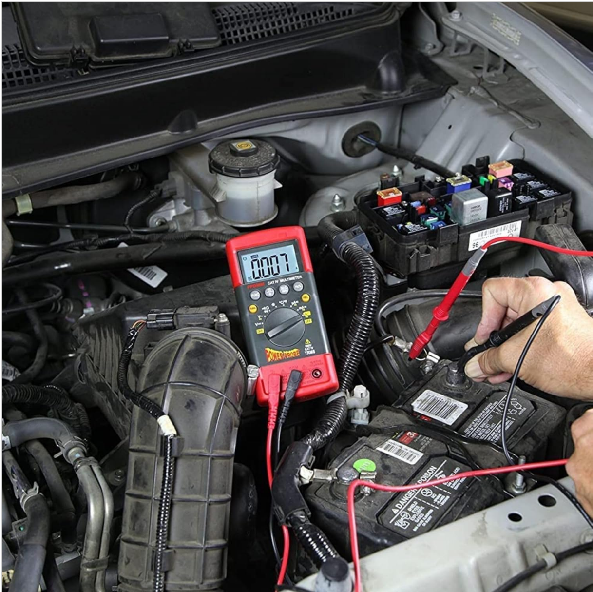
Figure 4.2: The Digital Multimeter displaying a voltage reading while connected to a car battery. The red and black test leads are attached to the positive and negative terminals of the battery, respectively.
