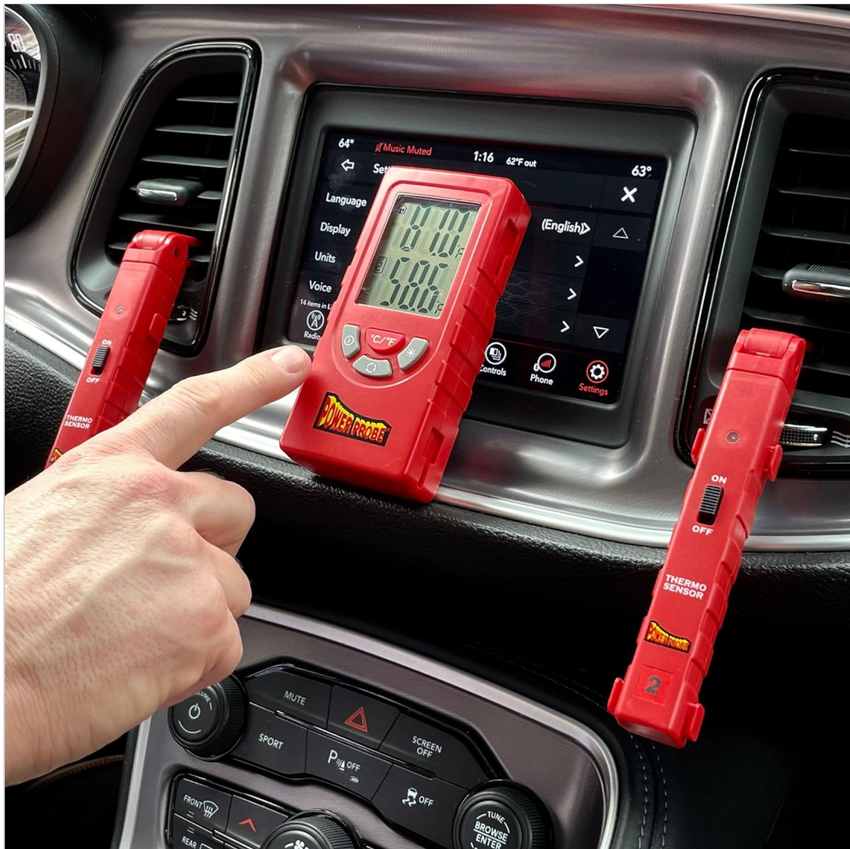
Figure 4.4: The main display unit of the Auto AC Temperature Testing Kit positioned on a car dashboard, showing dual temperature readings. Two wireless sensors are visible, one placed in an AC vent and another held by a hand, demonstrating multi-point temperature monitoring.
