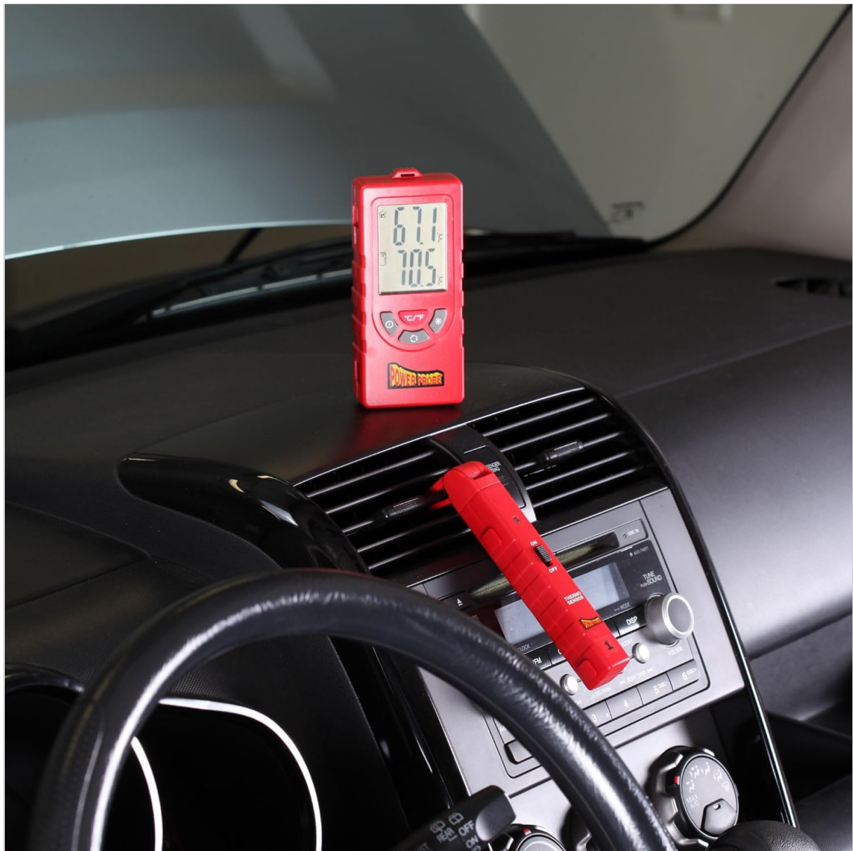
Figure 4.3: A wireless temperature sensor from the Auto AC Temperature Testing Kit inserted into a car's air conditioning vent, displaying a temperature reading on its screen.
