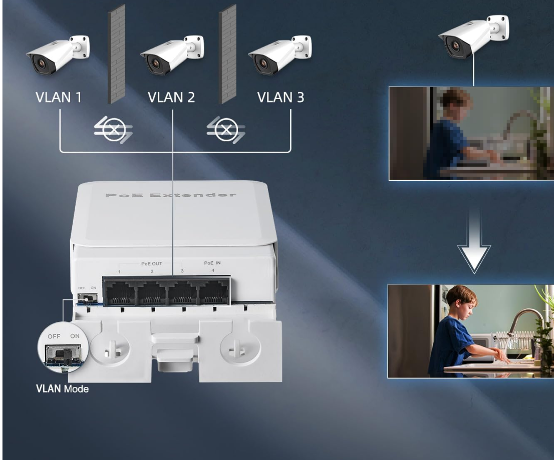
Image: Diagram illustrating the VLAN mode dipswitch and how it isolates traffic between connected devices (VLAN 1, VLAN 2, VLAN 3).
