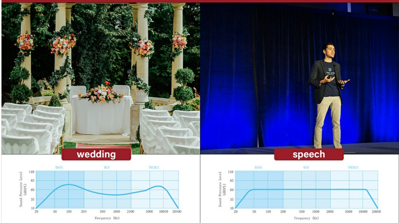
Image: Visual representation of DSP settings for 'Wedding' and 'Speech' modes, showing their respective frequency response curves.
