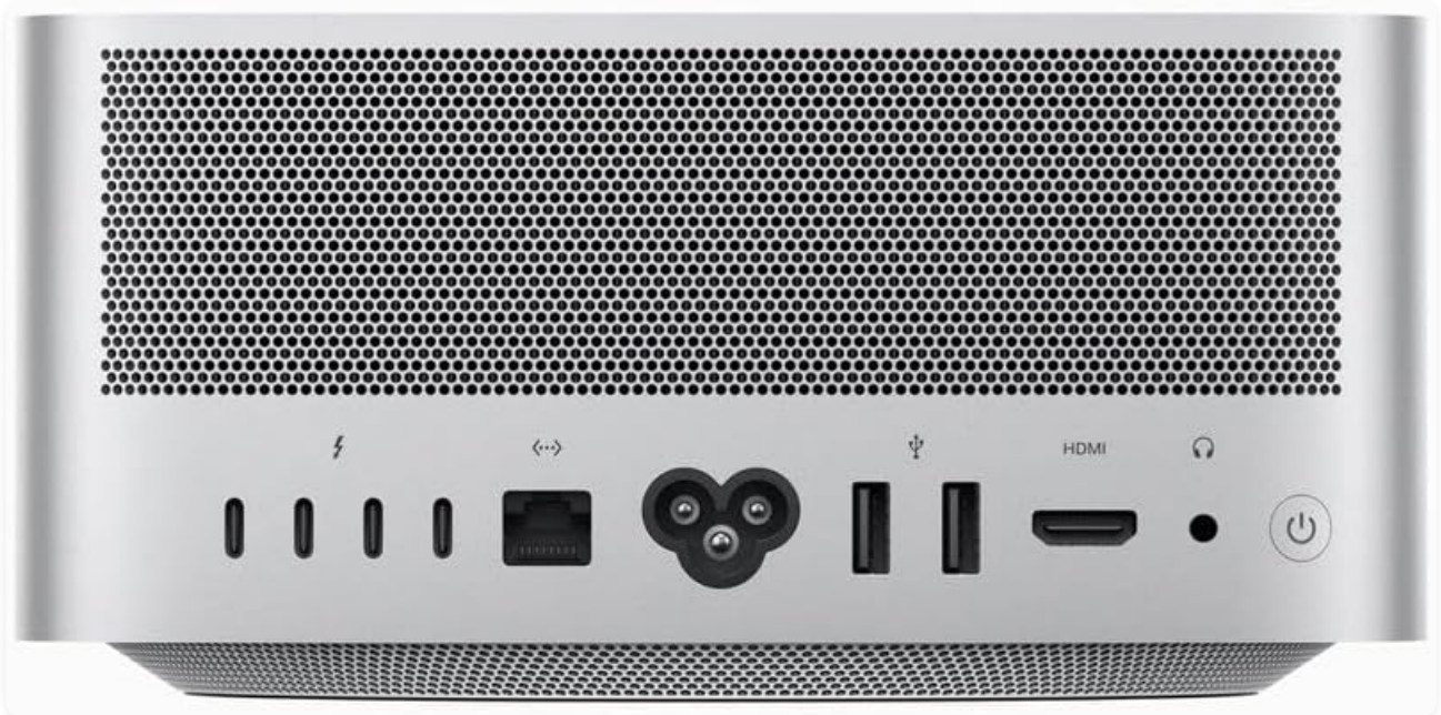
Image: Rear view of the Mac Studio, displaying the four Thunderbolt 4 ports, 10 Gigabit Ethernet, power input, two USB-A ports, HDMI, and a high-impedance headphone jack.
