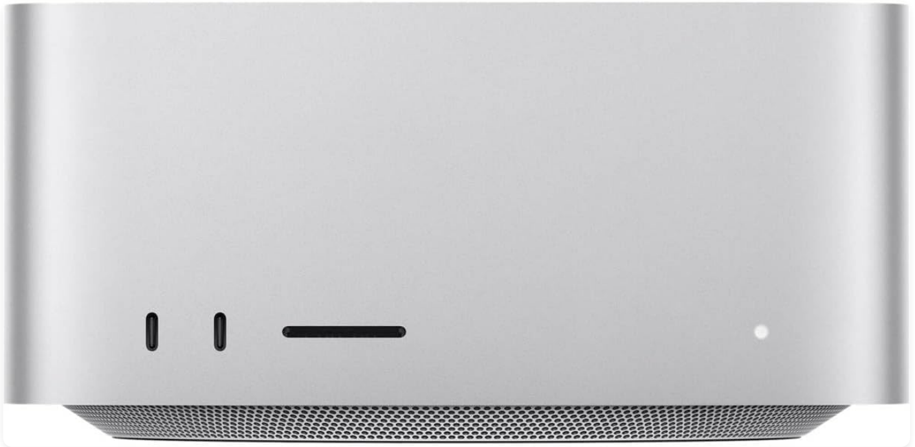
Image: Front view of the Mac Studio, showing the power indicator, SD card slot, and two USB-C ports.
